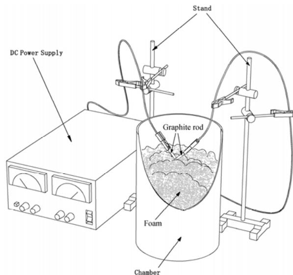
FIG. 1: Schematic of the experimental setup for MWNT preparation by the DC arc discharge method in foam.
