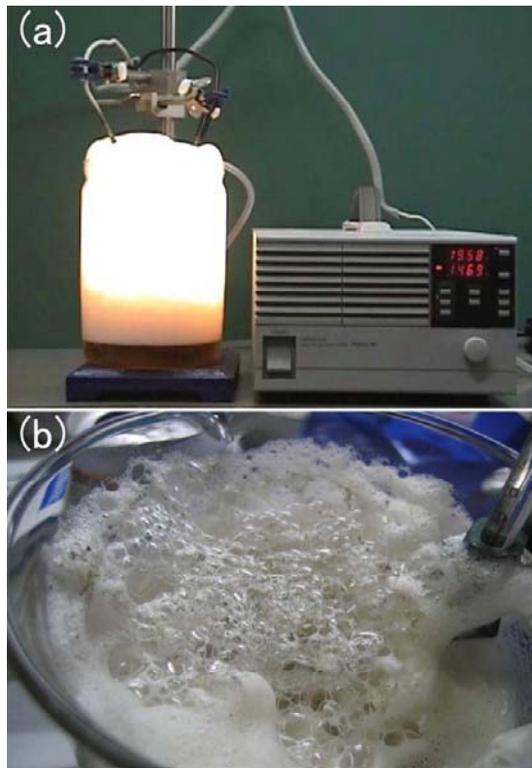
FIG. 2: DC arc discharge in foam: (a) Arc discharge in foam; (b) Surface of the foam after DC arc discharge.
