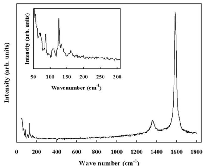
FIG. 5: Raman spectra of CNT cluster produced by arc discharge in foam.
