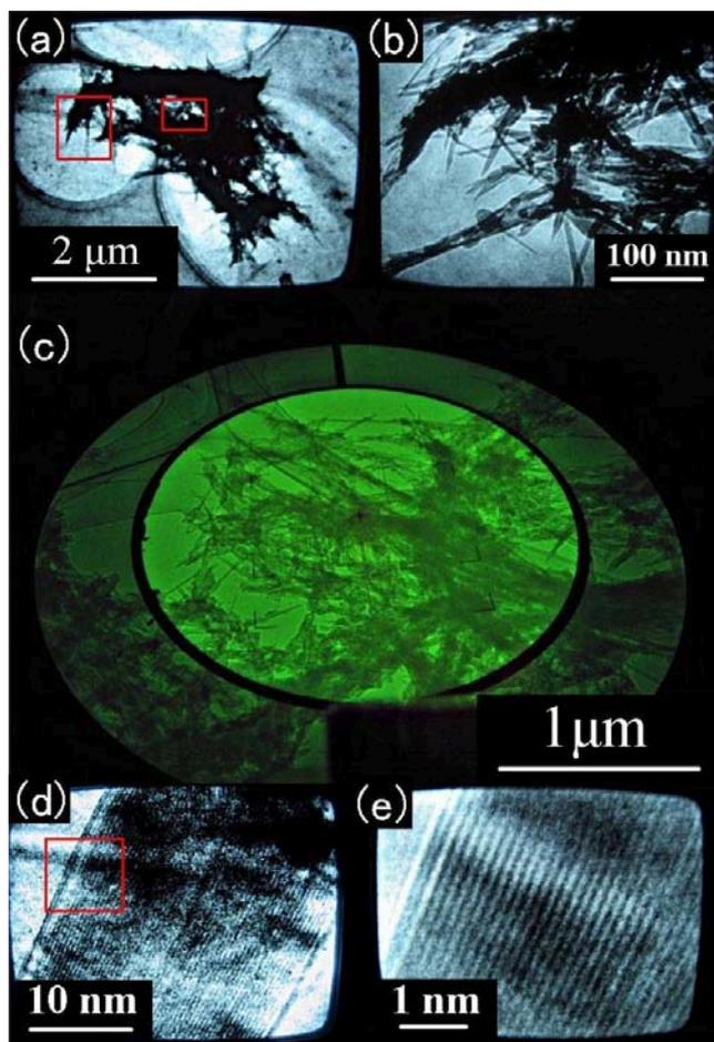
FIG. 4: TEM images of fine particles on the foam surface: (a)-(c) low-magnification views; (e) high-magnification view of (d).
